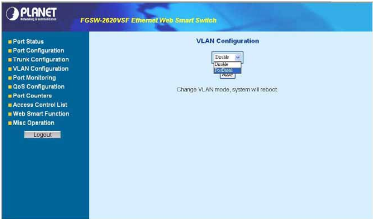
Figure 4-27 Disable Port-based VLAN function Web Page screen
